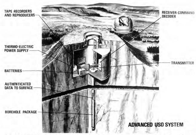
BOREHOLE PACKAGE would be emplaced at depth of 1500 or 2000 teet in b-inch diameter noie. Seismic detectors would be either force balance or quartz fiber torsional accelerometers.
